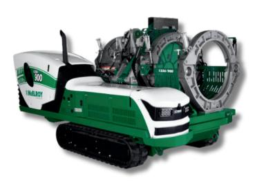
TThe McElroy TracStar® 900 Series 2 Automatic is a self-contained, selfpropelled, all-terrain fusion machine with an on-board generator for powering the heater. It is hydraulically powered to assist all fusion functions including the operation of the jaws, pipe lifts, heater and facer. The machine is capable of fusing 340mm to 900mm (12" IPS to 36" OD) thermoplastic pipe in accordance with many of the international fusion standards.
