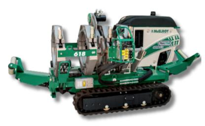
Drawing on insights directly from users in the field, the TracStar® 618 Series 2 has undergone a comprehensive redesign. It now utilizes the same base vehicle as the TracStar 250 and 412 models, boasting a robust diesel engine. This feature is particularly advantageous on job sites where the use of gasoline is restricted.
