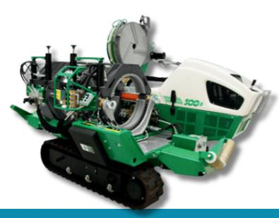
The McElroy TracStar 500 Series 3 is engineered to butt fuse pipes ranging from 6 inches IPS to 20 inches OD (160mm to 500mm). Launched in 1997, the original TracStar 500 broke new ground as the first self-contained, self-propelled, allterrain machine designed for fusion tasks, setting a high standard for the McElroy lineup.
